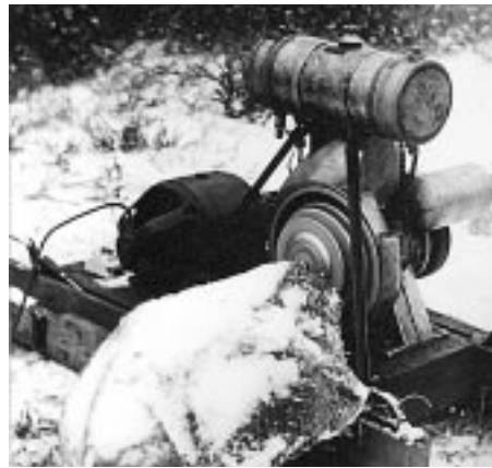
An early power source - the motor generator "Elsa".....
