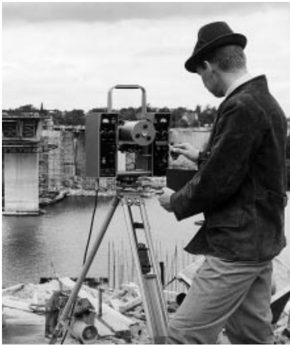
Geodimeter Model 6 was used for surveying the Essingeleden highway bridges in Stockholm.
