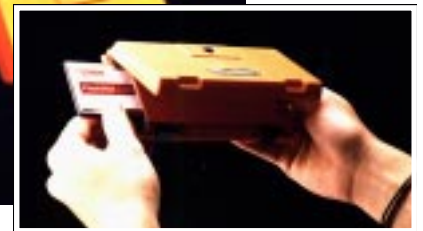
Geodimeter System 600, the Card Memory unit and the PCMCIA card for data storage.
