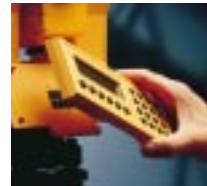
Constructor 100 features a detachable keyboard/memory unit.
