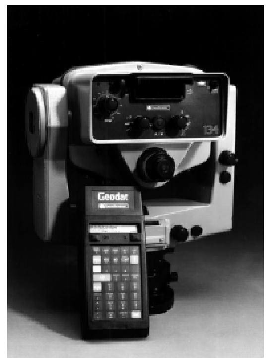
The control unit of Geodimeter 700 mounted on Geodat 700 data collector
